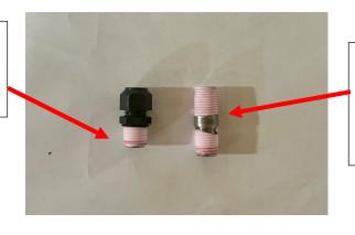
Put Teflon on the stainless-steel nipple only if the installation corresponds to #2.
