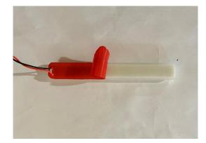
Glue the LED to the cleaned surface, in the previously chosen location. Press firmly on the LED to ensure that it is well glued. Then, pass the wire through the ¼ hole.
