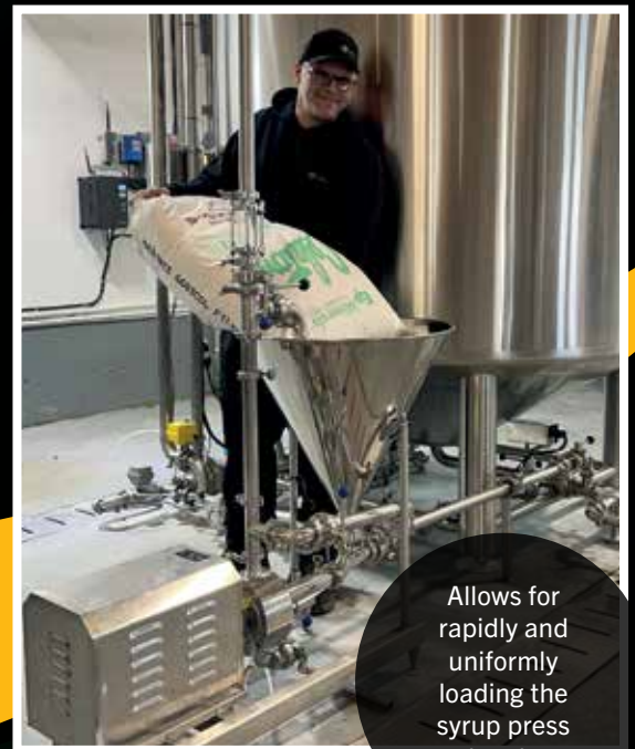
Dynamic Mixer YRL 1-100 with 5.5 HP motor 668429
